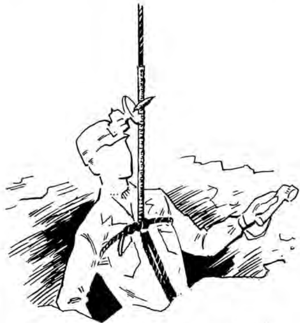
Greenfield flexible conduit protecting rope from flame of carbide lamp.
